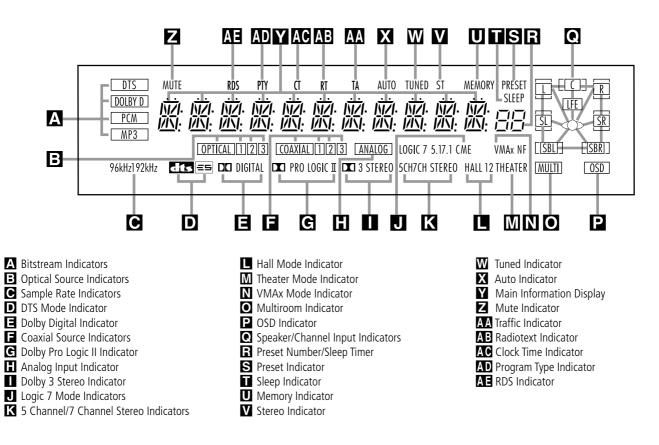
A Bitstream<sup>™</sup> Indicators: When the input is a digital source, one of these indicators will light to display the specific type of signal in use.
